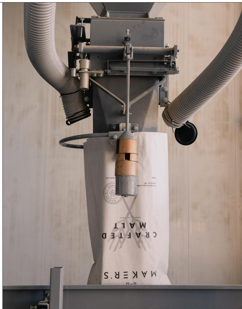
A 25-kilogram malt bag is filled at the Maker's cleaning and bagging facility. Craft brewery clients value experimentation, variety, freshness and local availability.
